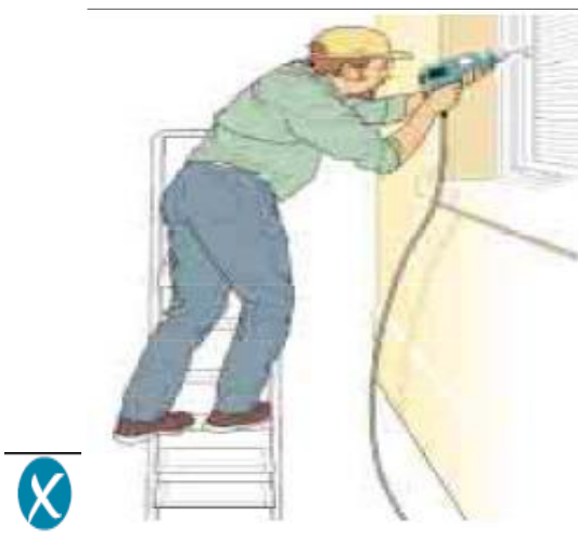
Incorrect – steps side on to work activity
